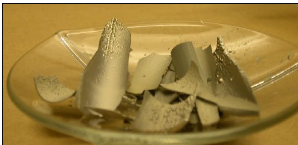
Figure 6. Brittle segments of pure nickel removed from the decomposer cell.
