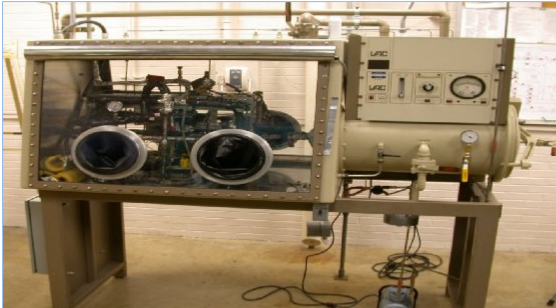
Figure 3. CVMR® Separation unit installed in a B&W glovebox at LTC.
