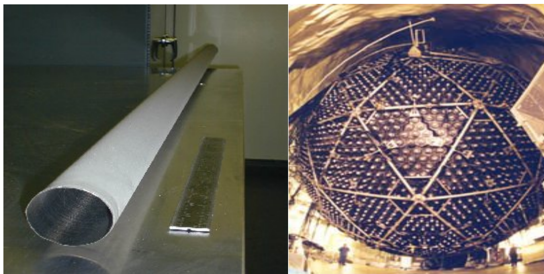
Figure 1. For the SNO project, CVMR ® used a precision, ultra-pure nickel tube for SNO project and the final assembly of the detector for detection and characterization of neutrinos.
