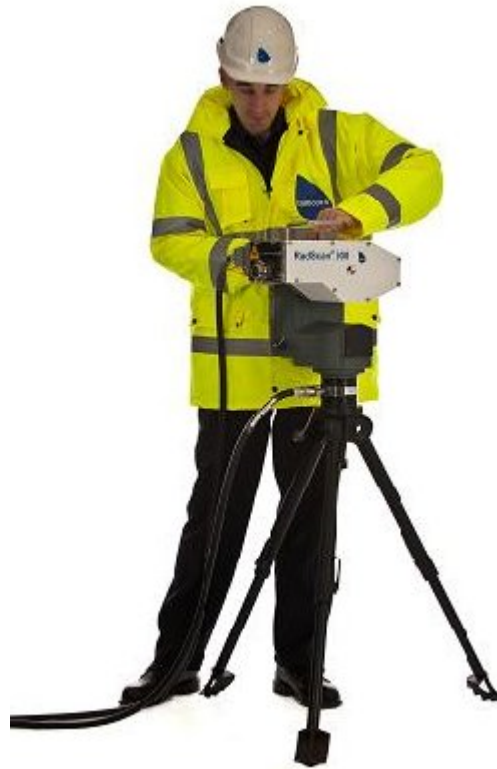
Fig. 3. A photograph of the RadScan gamma-ray imaging system.
