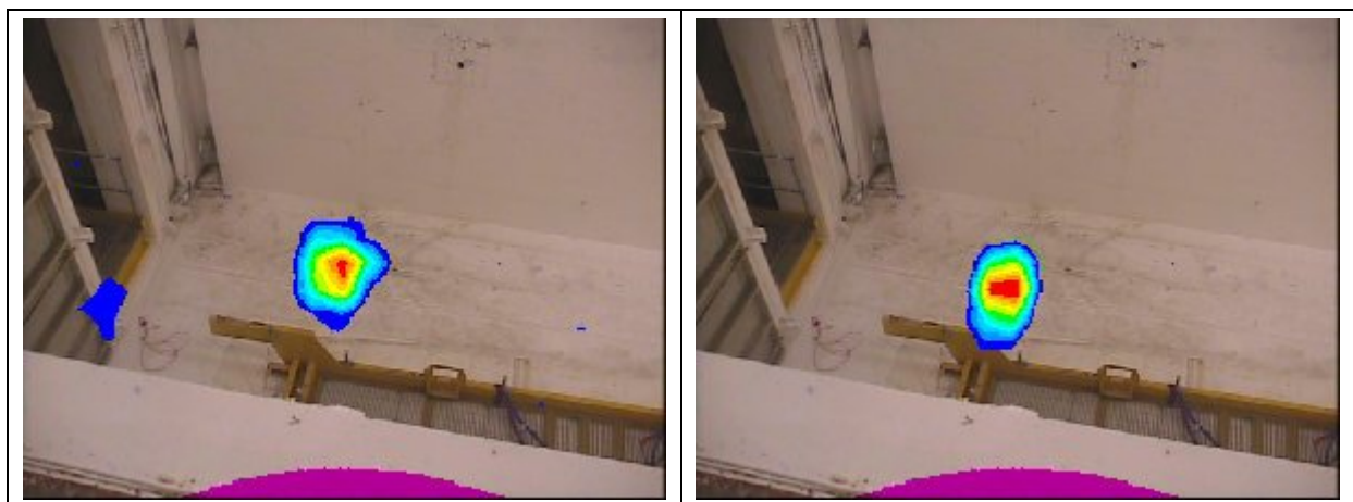
Fig. 8. Detail of the most intense hotspot in the South Main Pond shown for Co-60 (left image) and Cs-137 (right image).
