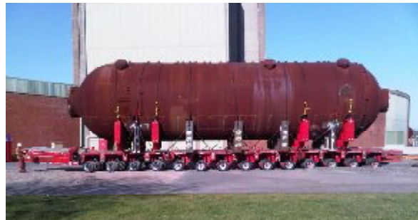
Fig.4 Photograph showing boiler loaded onto SPT
