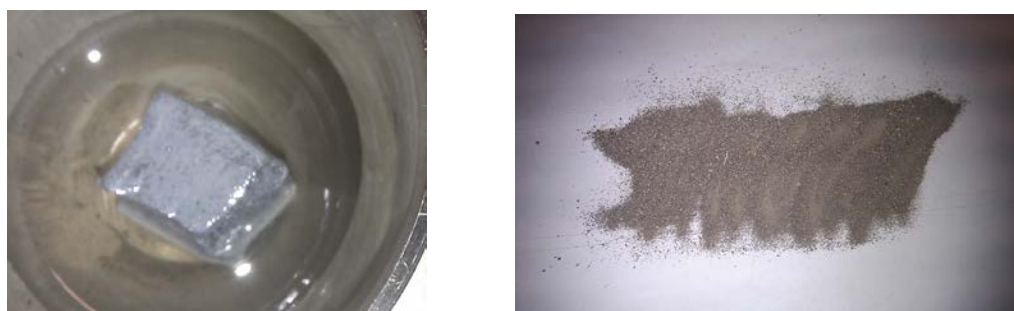
Fig. 4 Cerium metal before (ingot) and after heat treatment
