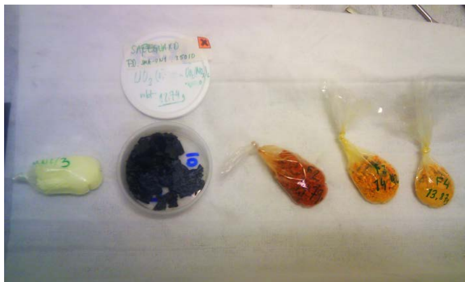
Fig. 3 Uranyl nitrate from untreated to pyrolysed under different conditions
