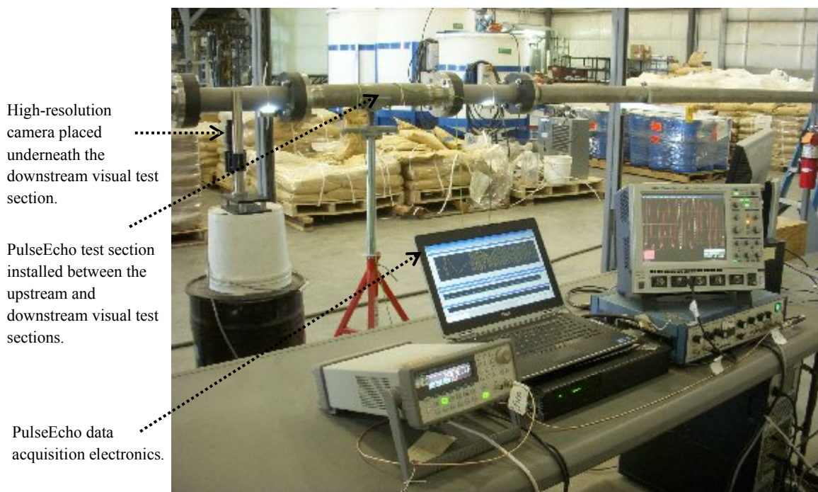
Fig 3. Photograph of the PulseEcho test section and visual test section installed in the WRPS RSD/Waste Feed Flow Loop.
