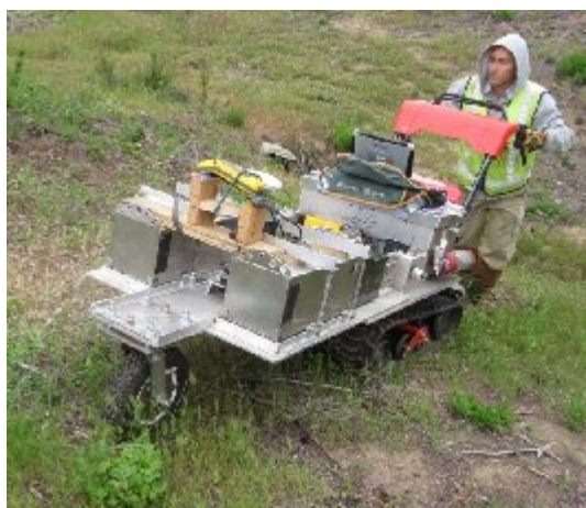
Figure 2: TMGS operator conducting a gamma scanning survey on a steep gradient.
