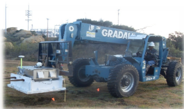
Figure 1: An ERGS II operator testing for proper scanning velocity before conducting surveys.
