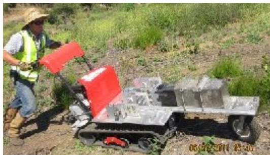
Figure 3: STGS operator conducting a gamma scanning survey on a steep gradient.
