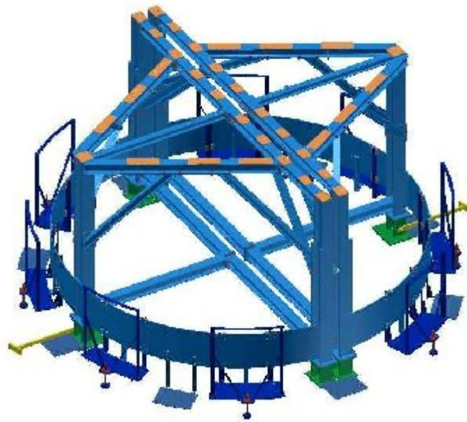
Figure 3 - Steam Dryer Support Stand
