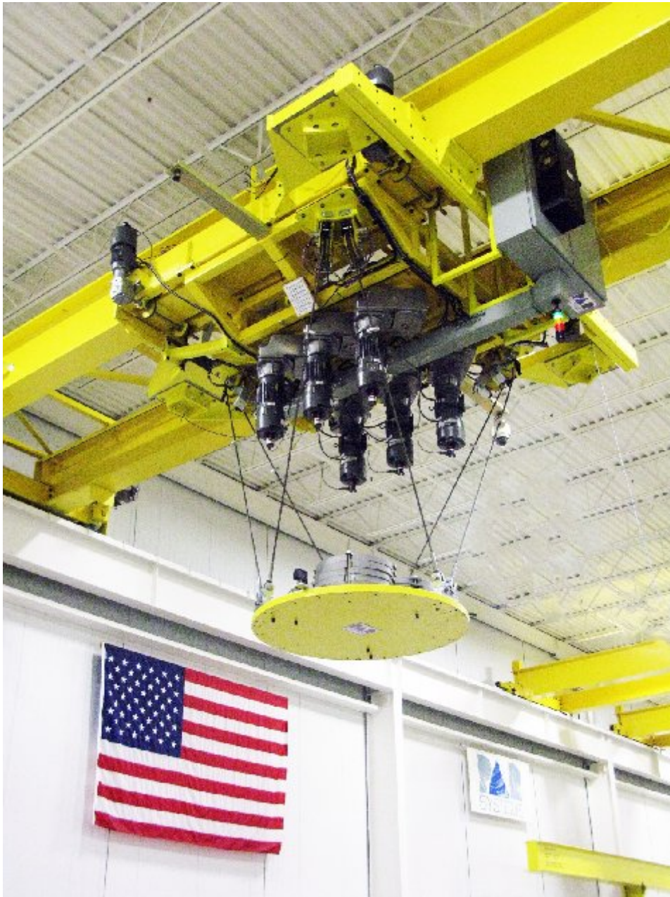
Figure 9 - 1/4 Scale Model of Tensile Truss - Fully Functional
