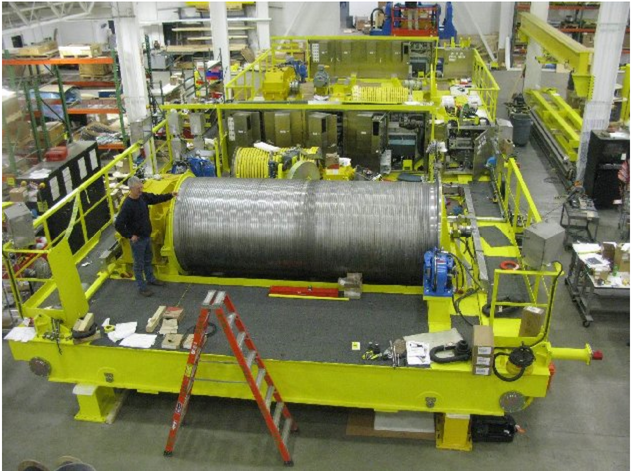
Figure 6 - Classic (front) and Secure (rear) Carriages during assembly, January 2013
