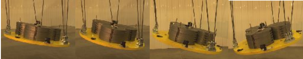
Figure 10 Scale Model Tension Truss Lower Platform - using hoist control to achieve various orientations
