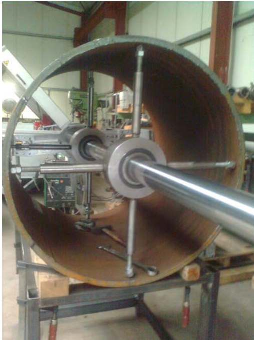
Figure 1: “overturning machine” with a sample pipe
