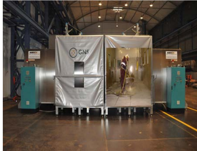
Figure 5: example of a blasting cabin
