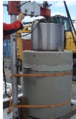
Figure 4: first trial with diamond core bit
