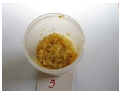
Fig. 3. Sample appearance after solidification of the vacuum oil. There was used No. 960 polymer, and proportion between polymer masses and liquid (S:L) was 1:5.
