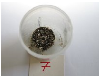
Fig. 2. Sample appearance after solidification of the residue from waste tank. There was used the mixture of polymer No. 910 (20%) and No. 960 (80%), and proportion between polymer masses and liquid (S:L) was 1:3. Total specific \alpha -activity - 6.61 \cdot 10^6 Bq/kg, total specific \beta -activity - 1.3 \cdot 10^8 Bq/kg.
