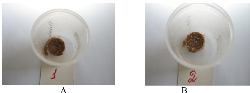
Fig.2. The appearance of the sample after solidifying the evaporator cube residue. The total \alpha -activity was 2.5 \cdot 10^6 Bq/kg; the total \beta -activity was 7.3 \cdot 10^7 Bq/kg.
