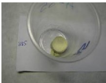
Fig.1. Final condition of the product from Sample No.385 – after solidifying the simulated solution with polymer No.960 and the additives of bentonite and silica sol solution of \text{SiO}_2 concentration of 95 g/L
