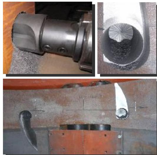
Fig. 7 HWZ drill rod during mock-up tests
