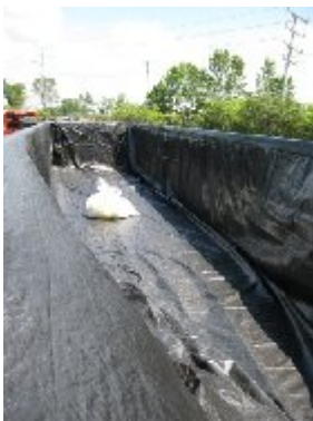
Figures 1 - 2: Lined railcar interior (left). Liner installation assisted by aerial lift (right).
