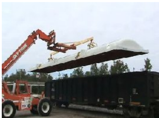
Figure 14 - 15: Placement with all-terrain forklift (left). Hard cover suspended from crane (right).
