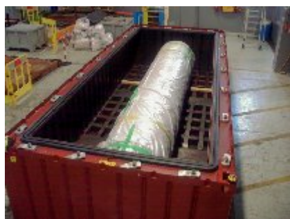
Fig. 11: Multi-Element Bottle (MEB) located within the isofreight container (left) and the assay equipment deployed at one of the measurement positions around the container (right).
