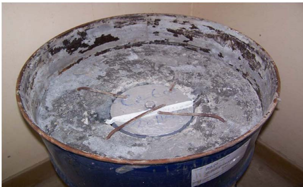
200 L DRUM CONTAINS THE PREFABRICATED CASK CONTAINS THE DISMANTLED CO 60 OR CS 137 SOURCES
