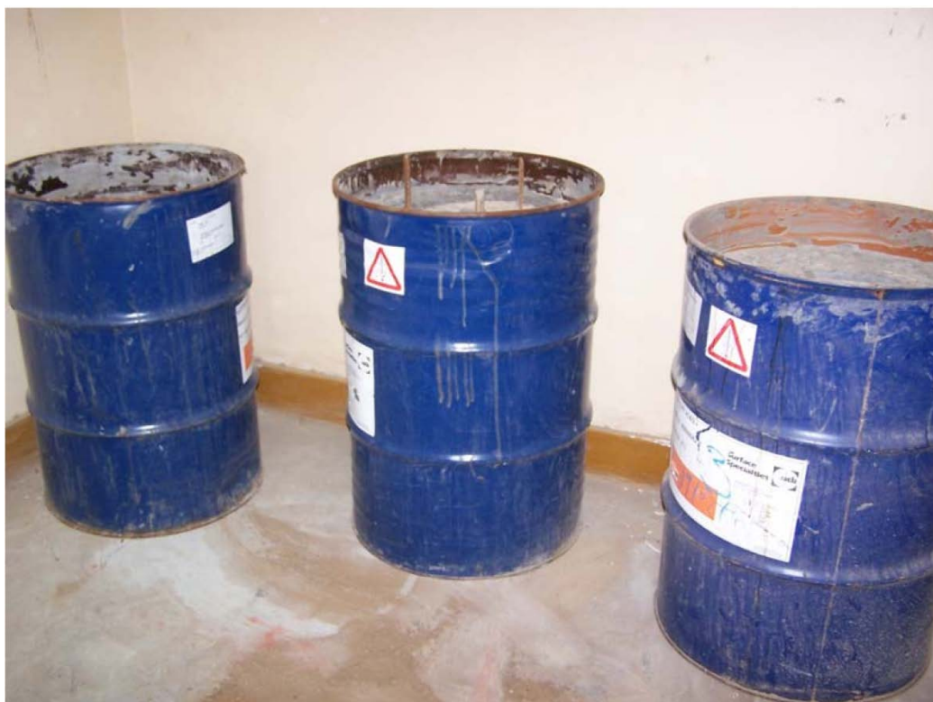
CONDITIONED DRUMS READY FOR INTERIM STORAGE
