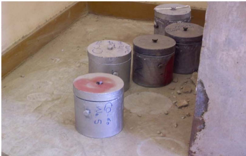
PREFABRICATED CASKS CONTAIN THE DISMANTLED CO^{60} OR CS^{137} SOURCES
