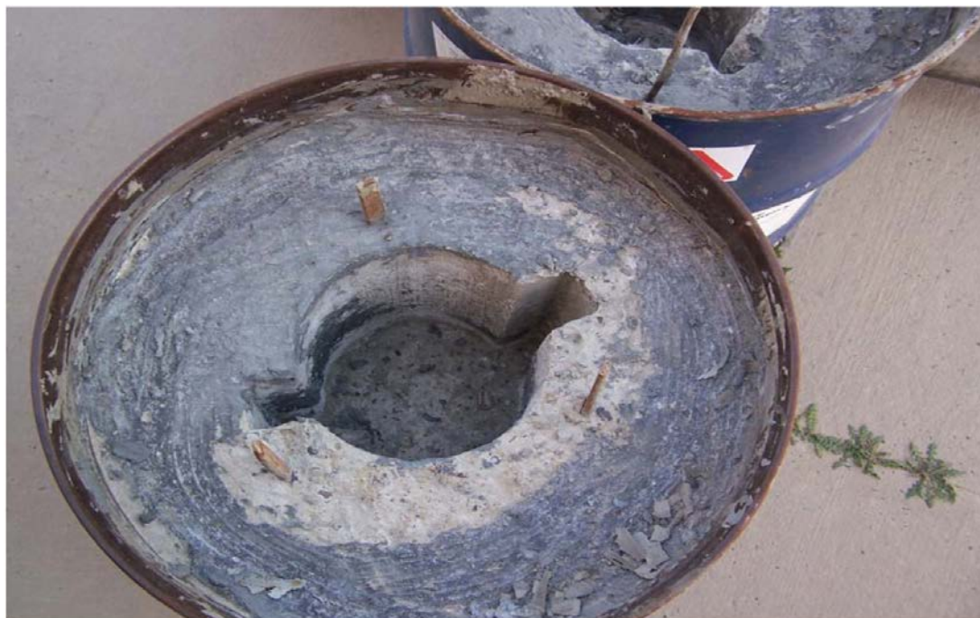
200 L DRUM READY FOR THE PREFABRICATED CASK CONTAIN THE DISMANTLED CO^{60} OR CS^{137} SOURCES
