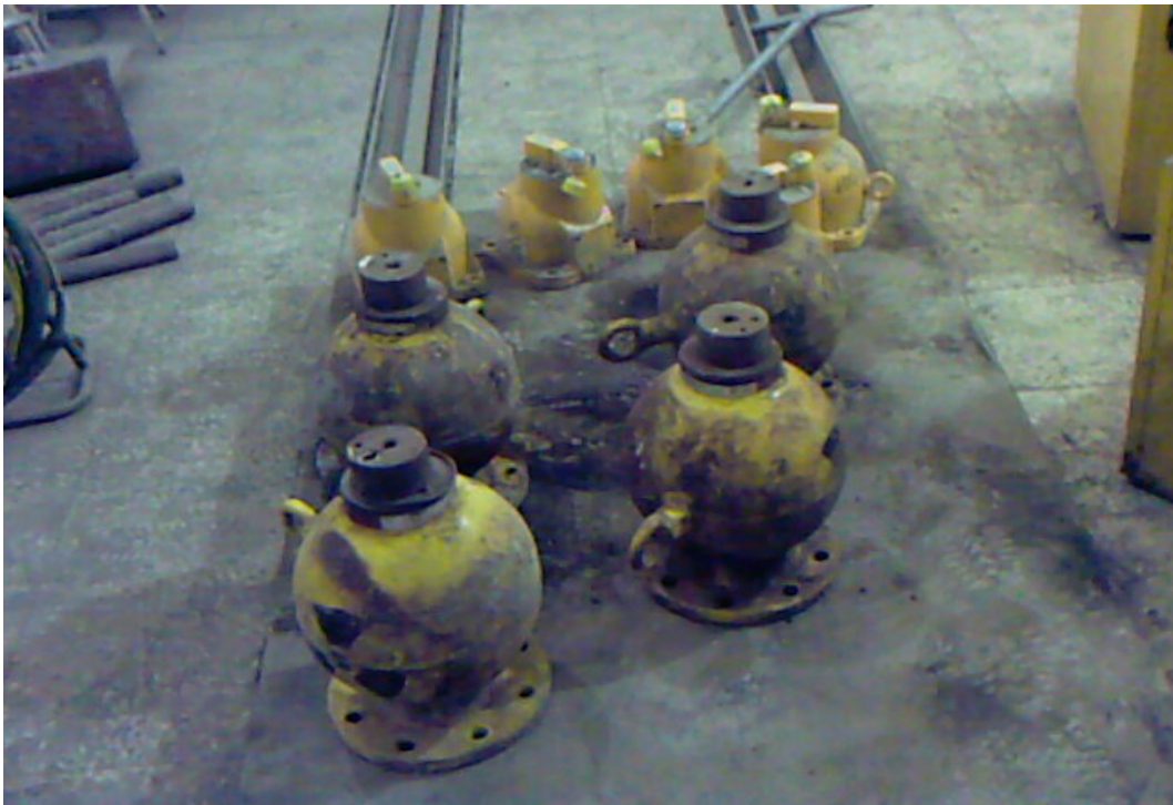
SPENT CO^{60} & CS^{137} SOURCES BEFORE THEIR DISMANTLING
