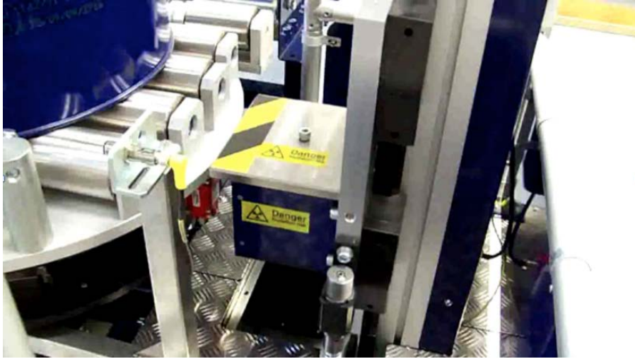
Figure 4. Tungsten shielded transmission source descending into the transmission source safe.
