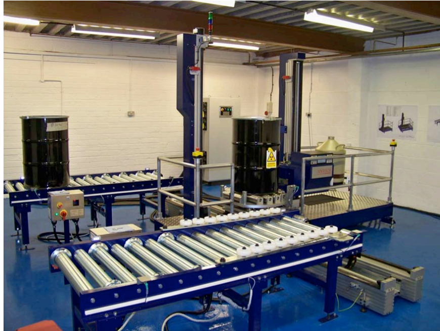
Figure 5. This is a photograph of the model G3250-3850-340 Wide Range SGS-TGS taken part way through a measurement during the FAT. Note that a drum is in the measurement position on the drum rotation platform. The transmission source is deployed and can be seen immediately to the left of the drum just above the mid-height. Another drum (from the previous measurement) is located on the output roller conveyor. The drum centering guides can be seen on the input roller conveyor in the foreground.
