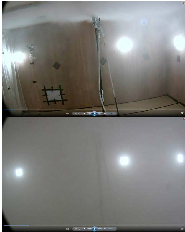
Figure 5 Images of the chamber after 10s and 90s fogging
