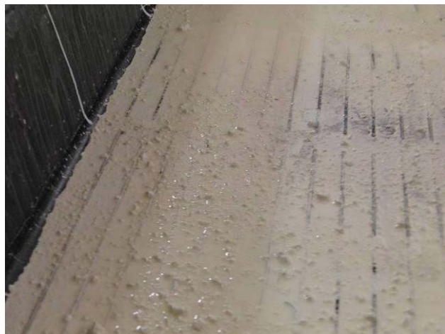
Figure 6 Tray of powder coated with FX1 during fogging chambers trials
