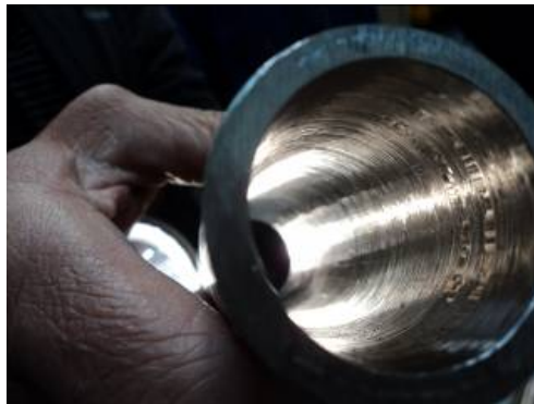
Figure 9: View of the internal part of a pipe, after milling
