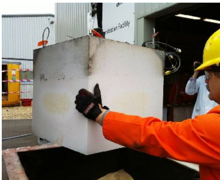
Figure 4. Inner ICV container being removed after test completion
