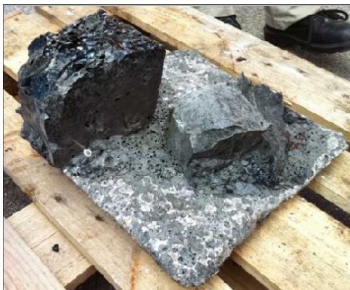
Figure 6 - Topside of Metal Phase with Two Glass Pieces Attached
