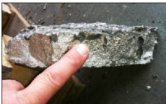
Figure 7 – Portion of metal phase showing dark spots
