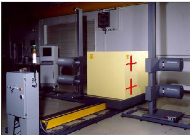
Figure 1. A common configuration of the Modular Box Counter is shown, consisting of two towers with two detector assemblies each and a conveyor system.
