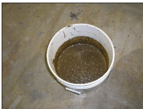
Figure 11. Wet, Spiked Soil Used for the Intermediate-Scale Testing.
