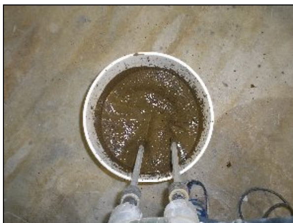
Figure 12. Intermediate-Scale Soil Sample during Simultaneous Treatment.
