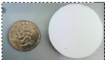
Fig. 5. A 7 x 40 mm-dia. test pellet pressed at 82 MPa controlled by wireless user interface.
