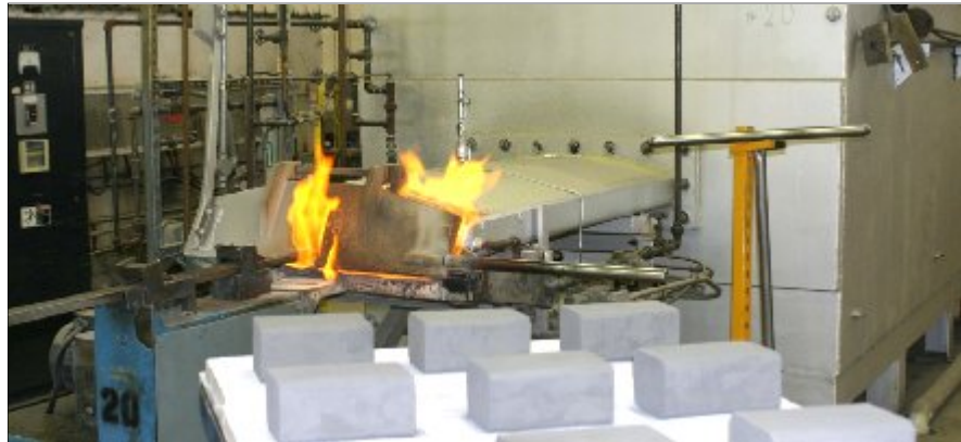
Figure 5. Pressed WHA powder compacts on ceramic media awaiting loading into hydrogen atmosphere stoker furnace. Total door-to-door time for a part on the order of 12 hours.
