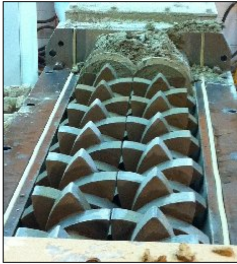
Fig. 2. Internal configuration of a Readco-Kurimoto, LLC continuous mixer, note the tight clearances between the intermeshing lens-shaped mixing paddles and the inside barrel diameter.
