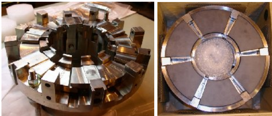
Figures 7 and 8 – Upper Radial Bearing and Thrust Bearing with and w/o Pads
