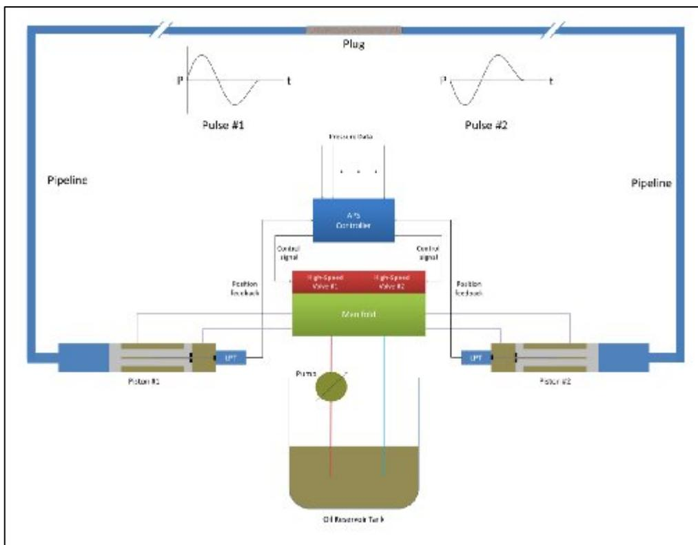
Figure 1. APS Schematic with major components labeled.
