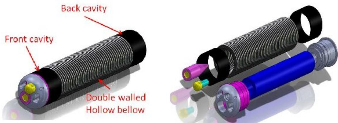
Figure 5. (a) Rendering of crawler, (b) exploded view of crawler assembly.
