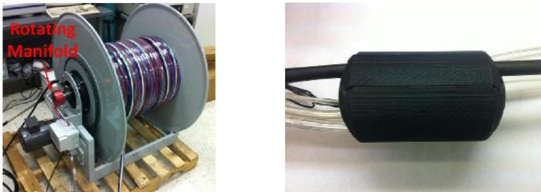
Figure 8. (a) Reel and tether assembly, (b) capsule manufactured from ABS.
