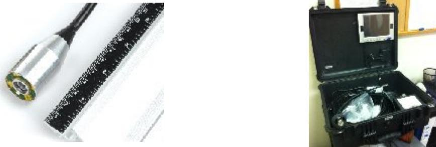
Figure 6. (a) Camera, (b) display station.
