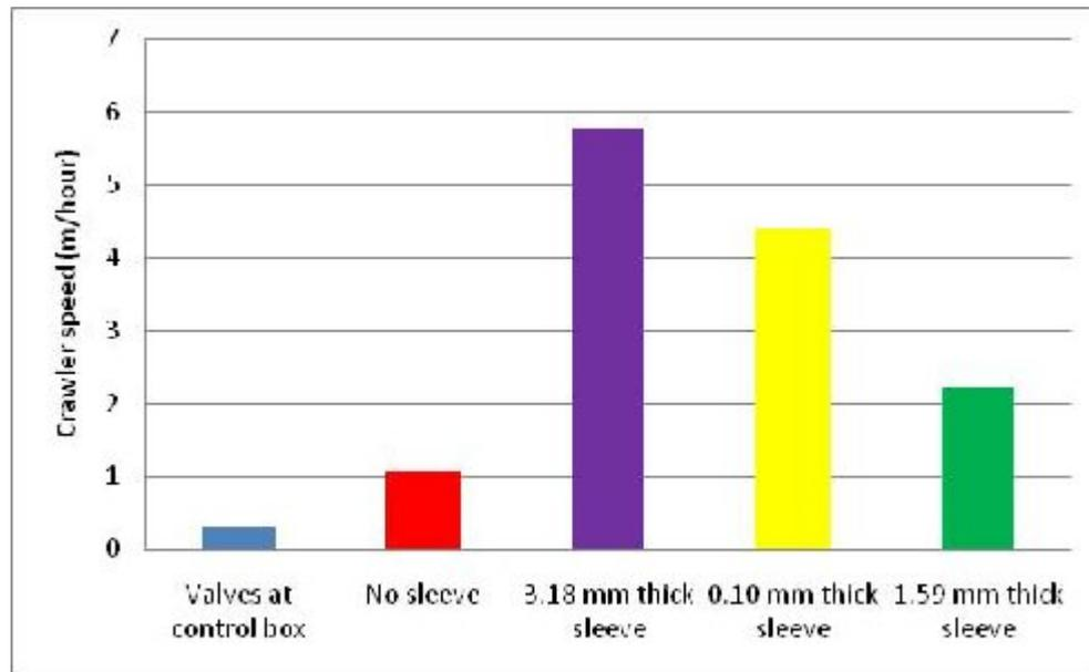
Figure 9. Speed of crawler using different sleeve configurations.
