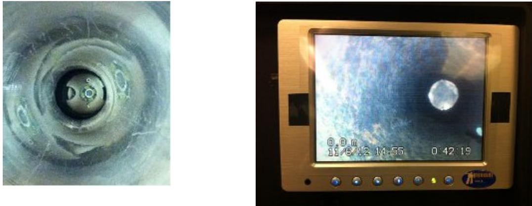
Figure 10. (a) Crawler navigating an elbow, (b) screen capture of carbon steel pipe section.
