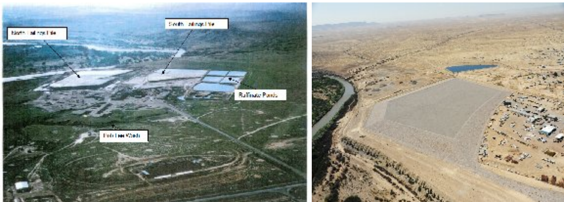
Figure 2 Aerial View of the Shiprock UMTRA Site in 1965 and after Completions of Disposal Cell in 1986 Disposal Cell
