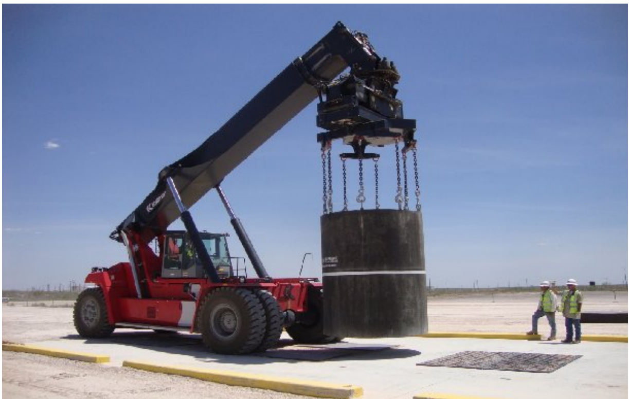
HD-MCC attached to the specialized Kalmar reach stacker at the WCS site.
