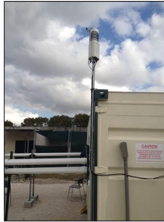
Figure 11. Weather station installed on the office container.
