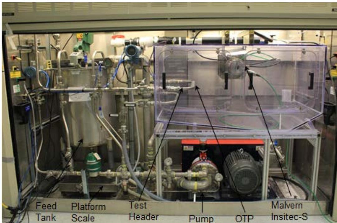
Fig 2. Small-Scale Test Loop
