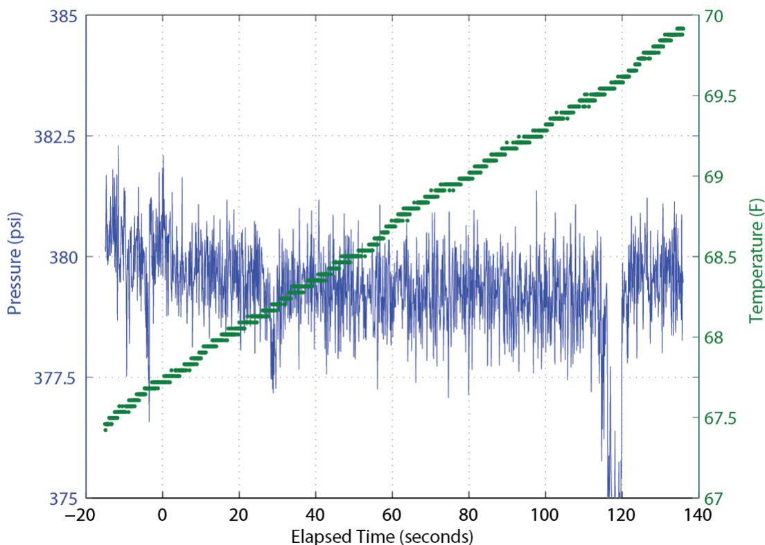
Fig 3. Pressure and Temperature Data for a 2-mm orifice at 2.6 MPa (or 380 psi) in water. An elapsed time of zero is approximately when the spray was initiated.
