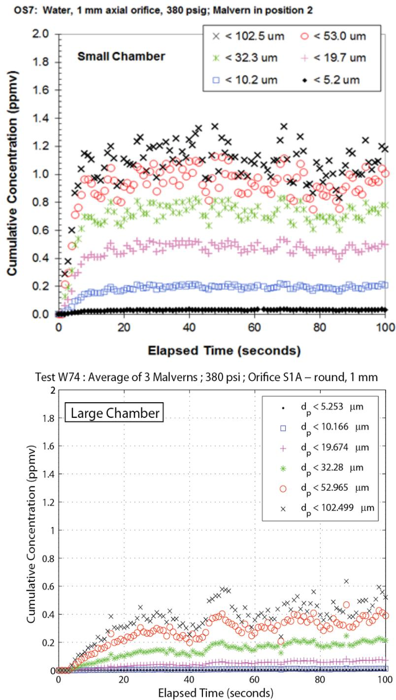
Fig 4. Comparison of the Transient Cumulative Droplet Concentrations in the Small and Large Chambers for 2.6 MPa (380-psi) Water Sprays from 1-mm Circular Orifices
