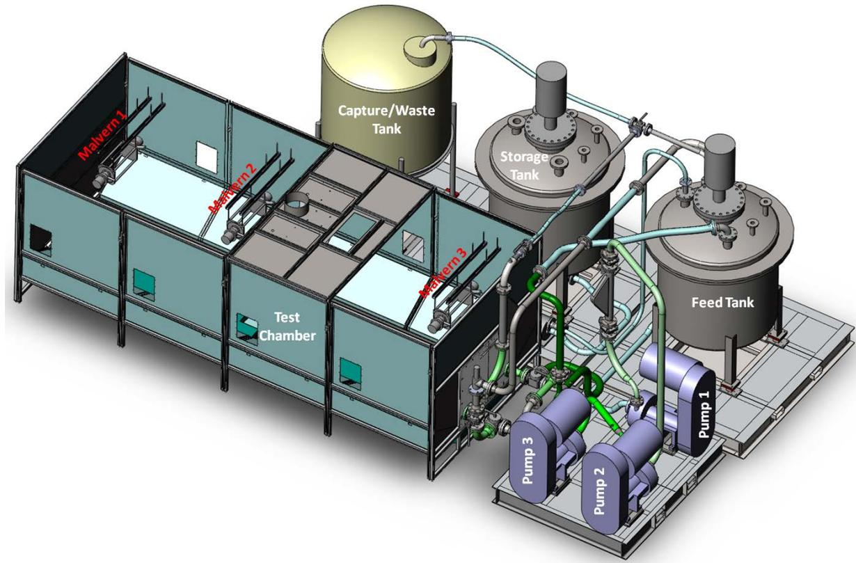
Fig 1. Schematic of the Large-Scale Test Stand
