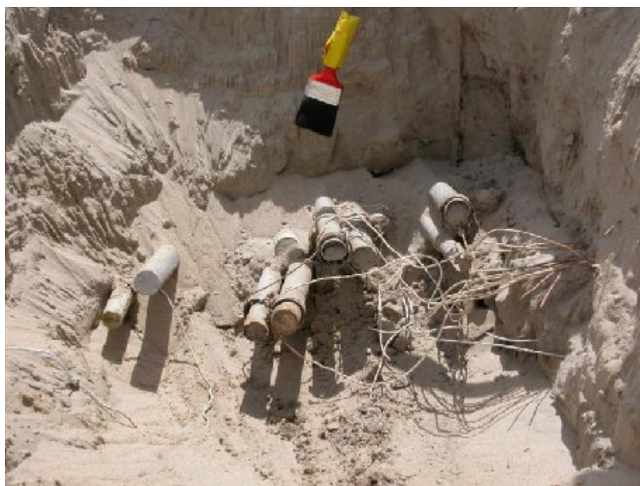
Fig. 3 Characterization activities in 2005 reveal the fuel rods. While several of the fuel rods or can had collars with identification tags, some fuel rods or cans were unmarked.
