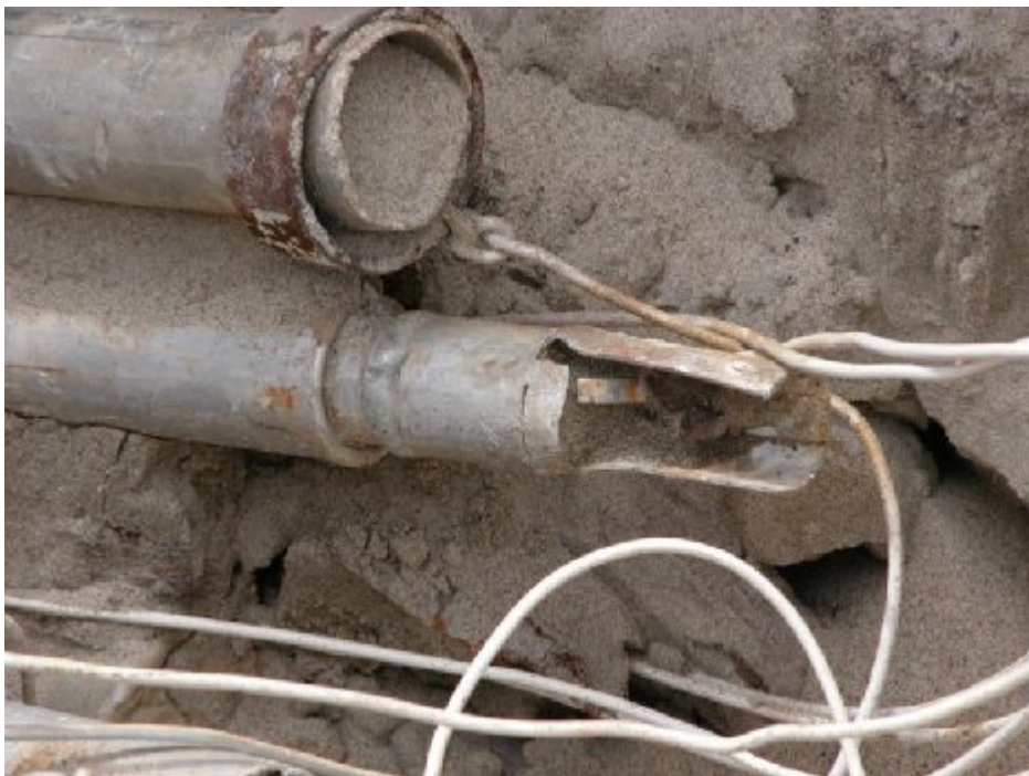
Fig. 5 A canned fuel rod that had been broken off inside a calandria tube.
