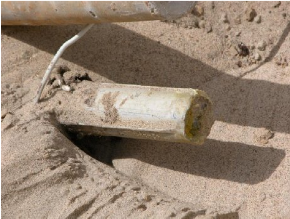
Fig. 4 An uncanned NRX X-rod which had been stripped of its flow tube, exposing the fuel sheath. Uranium corrosion is visually evident with the yellow product present.
