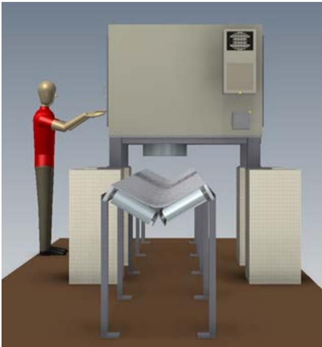
Figure 1, a drawing of the measurement system with the detector looking down on the conveyor belt.
