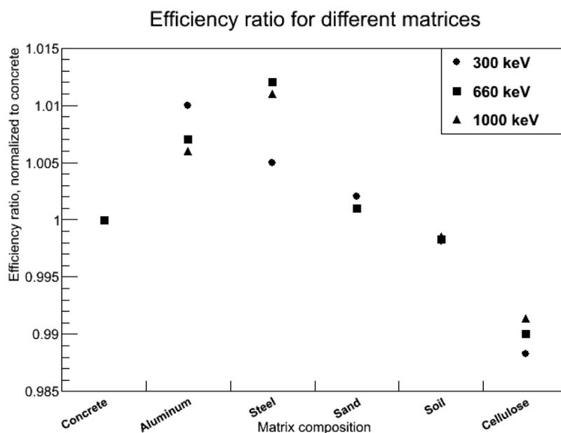
**Figure 3, the efficiency ratio of the six ash matrix compositions and concrete for 300 (circles), 660 (squares) and 1000 (triangles) keV.**
