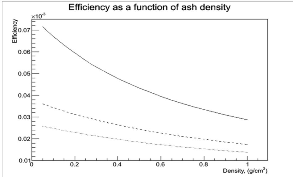
Figure 4, varying density keeping all other parameters constant for 300 (solid line), 660 (dashed line) and 1000 keV (dotted line).
