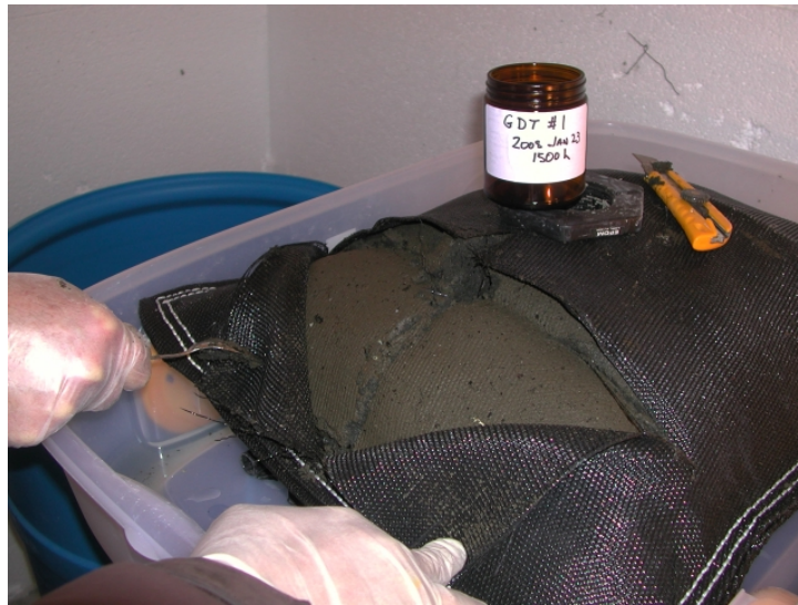
Fig. 3 Bench scale test of polymer additive and sediment containment bag dewatering system
