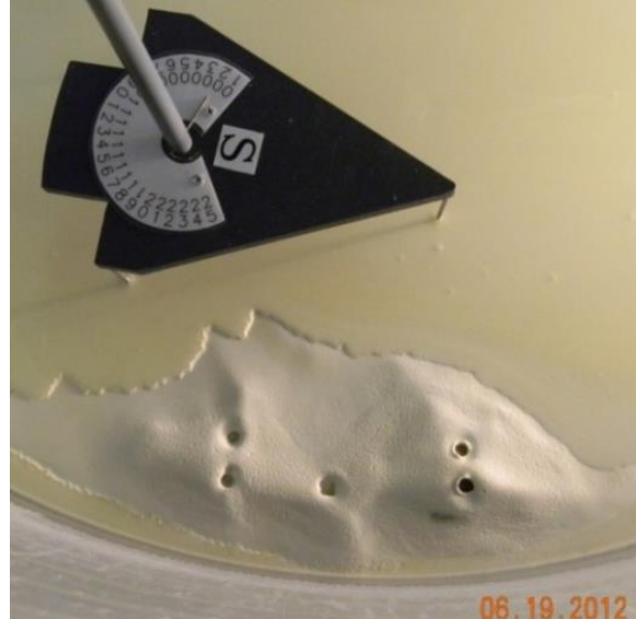
Fig.8. Triangular platform that stood 0.0762 m (3 in) off tank bottom. It also indicated which mound, e.g., S=South, and the tank level by manually setting indicator.
