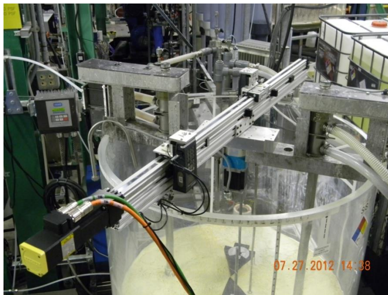
Fig. 6. Mechanical positioner in operation as the laser rangefinders map the bottom of the tank.
