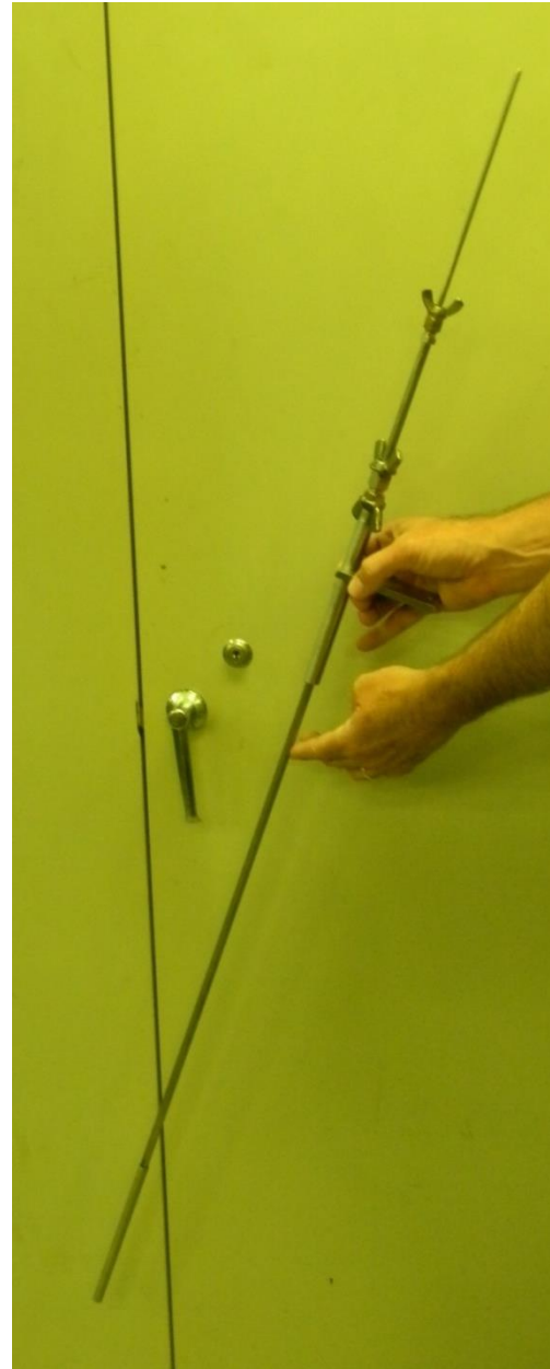
Fig. 13. Details of the core sampler (a) Illustrated drawing, (b) actual device.
