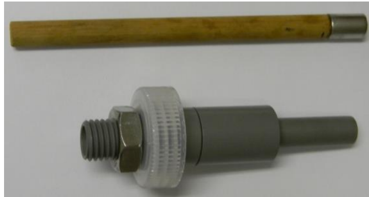
Fig. 5. Magnetic Separator (a) Photograph showing is 50-mm height, (b) As-built drawing. An aluminum reinforcing plate is not shown to better illustrate the device.
