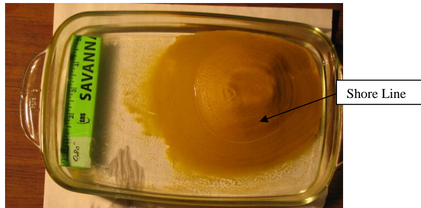
Fig. 10. Yellow sand mound in water to determine contrast between liquid and solids and estimate measurement uncertainty.
