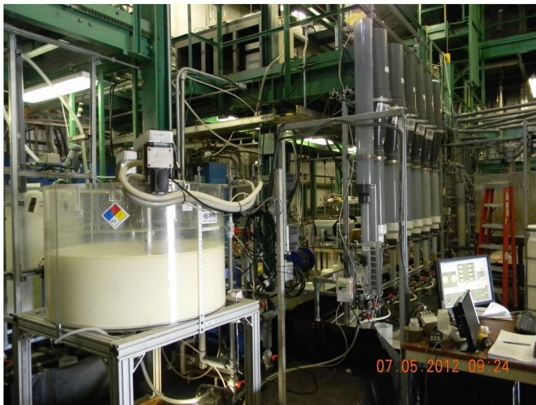
Fig. 1. The SRNL 1/22-scale Mixing Demonstration Tank with its 7 batch receipt tanks.
