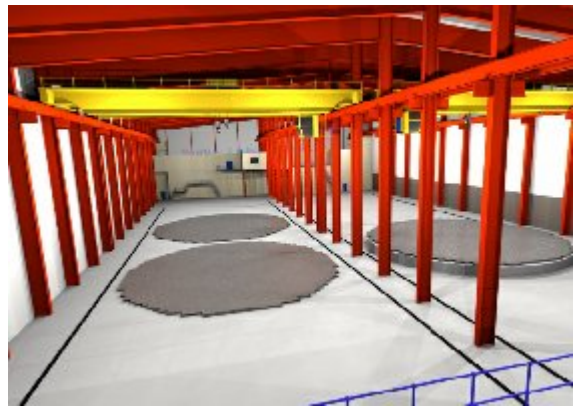
Figure 17 – Main hall of the DSU Enclosure with space to perform SNF retrieval and repacking into new canisters
