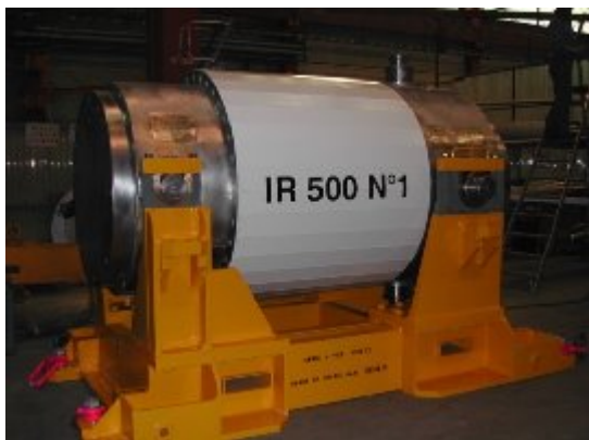
IR500 cask on its base, without the cover
