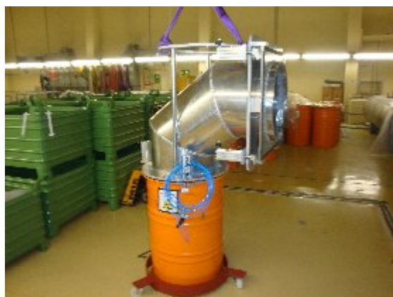
Fig. 3. Locking adapter with waste drum
