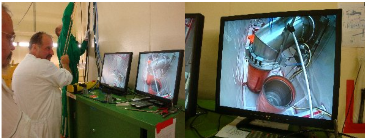
Fig. 4. Remote controlled filling of waste drums via locking adapter
