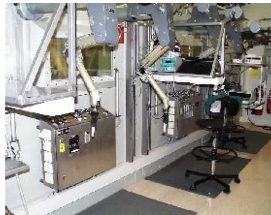
Fig. 2. Front side of the shielded boxes with hand operated manipulators
