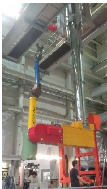
Fig. 6. Telescope and power manipulator during functional testing
