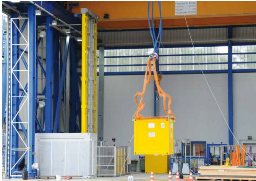
Fig. 2. Packaging drop test (LLW container at BAM Test Site Technical Safety)
