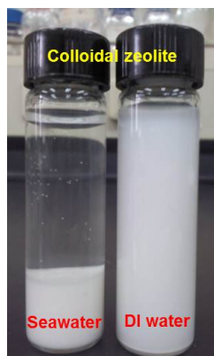
Fig. 2. Picture showing the different dispersion properties of colloidal zeolite in seawater and DI water.
