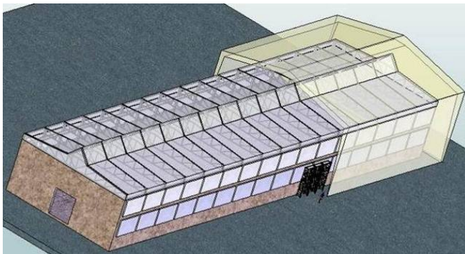
Fig. 4. Three-dimensional sketch of the building and airlock
