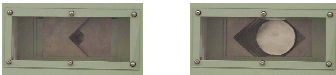
Figure 3. The TGS variable collimator showing minimum (left) and maximum (right) apertures.
