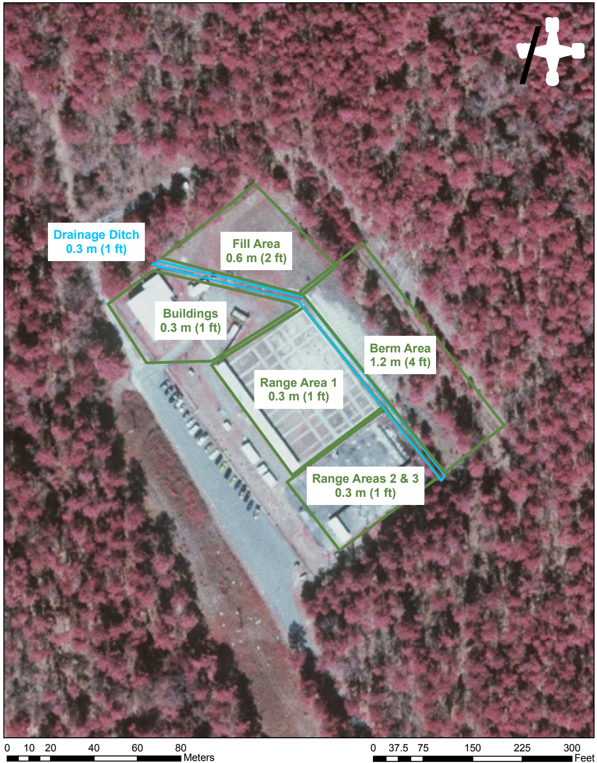
Figure 8. Soil Removal Area at SATA
