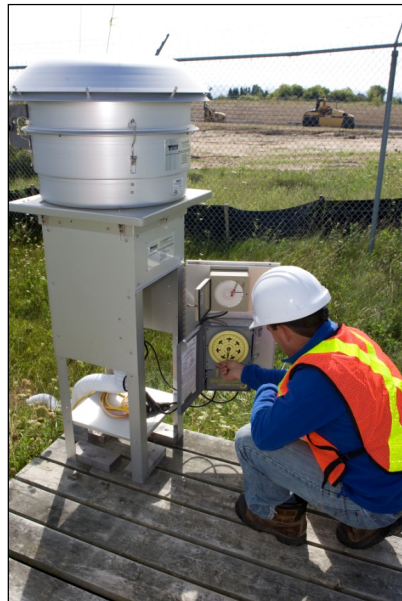
Figure 2: PHAI MO air monitoring Left: Hand-held real-time dust monitor Right: High volume air sampler at site perimeter
