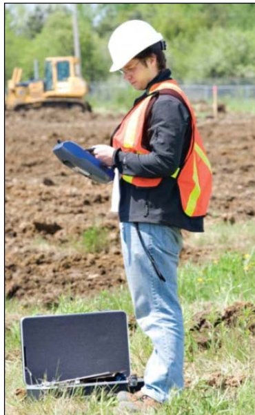
Figure 2: PHAI MO air monitoring Left: Hand-held real-time dust monitor Right: High volume air sampler at site perimeter
