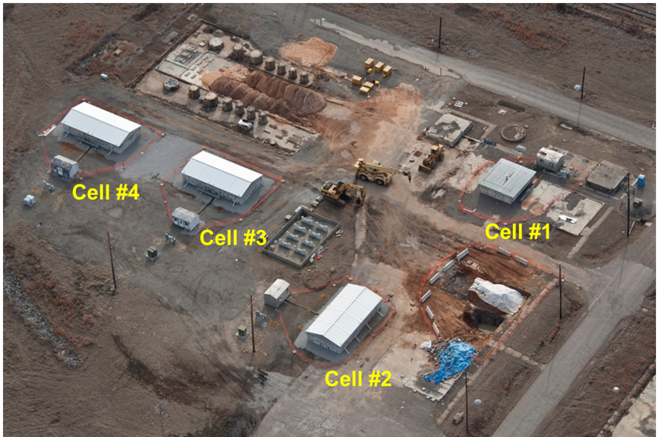
Figure 6: Thermal Detritiation Units used to remove tritium from concrete rubble and soil.
