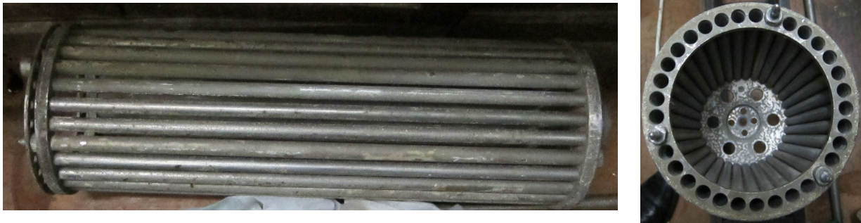
Fig. 6. Irradiation Basket with Tubes originally containing the Radiation Sources, Left: Side View, Right: Top View
