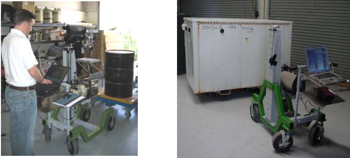
Fig. 1. Example of Portable Non-Destructive Assay System using Far-Field High Resolution Gamma Spectroscopy
