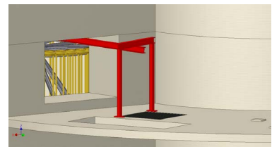
Fig 7. Carousel plant removal gantry
