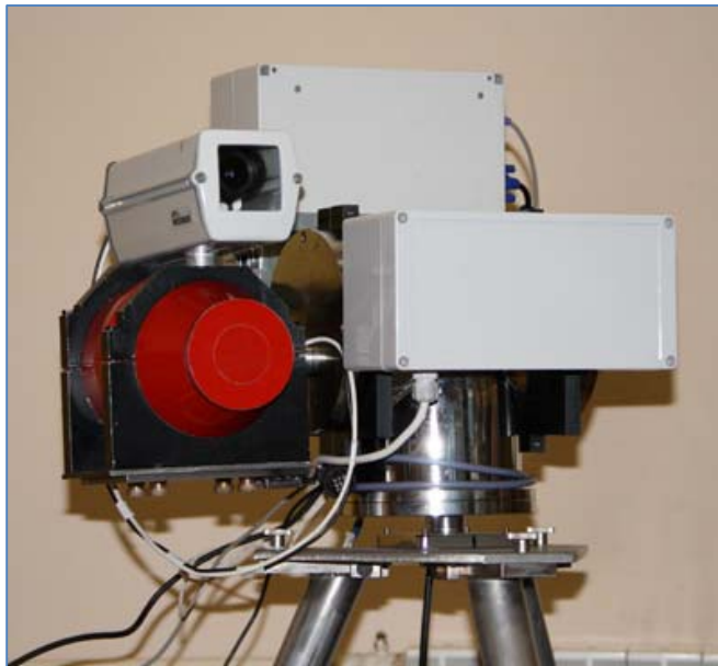
Fig.3. The remotely operated portable spectrometric system.
