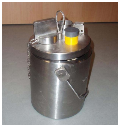
Fig. 11. 2-liters canister for storage of irradiating fragments
